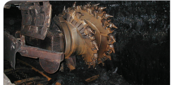
Longwall mining equipment shut down because of filtration issue.
